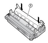
**5** Turn the two levers (1) on the toner cartridge firmly.
